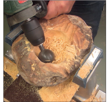
The larger model OrbiCut 40 on a hand drill.
